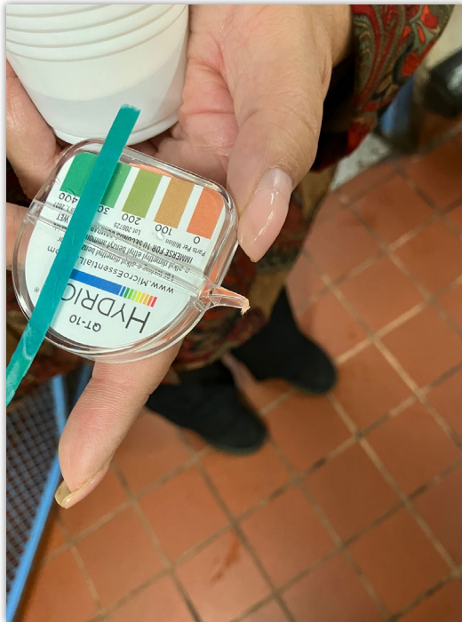
Photo 7. Chemical test strip showing high concentration of sanitizer. Source: OIG audit staff.
