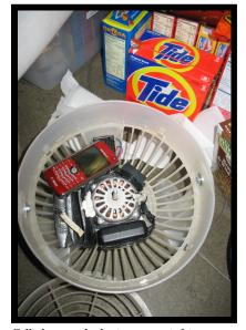
Cell phone and adaptor connected to electric desk fan motor to charge battery.
